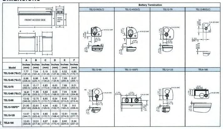
Note: All dimensions are for reference only. Lug & hardware dimensions not included. Batteries to be mounted with 0.5 in. (12.5 mm) spacing minimum allowing free air ventilation. Contact a C&D Representative for additional dimension information.\*(SLC) battery includes cable assembly. \*\* TEL12-105FS is a Front Access Battery and includes rope handles.
