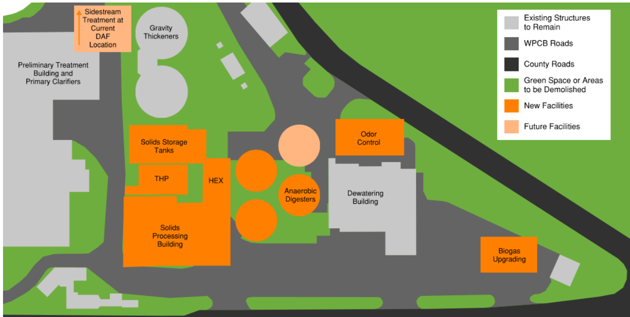
Figure 17-2. Option 2: Decommission Existing Dewatering Building—Alternative Concept 1
