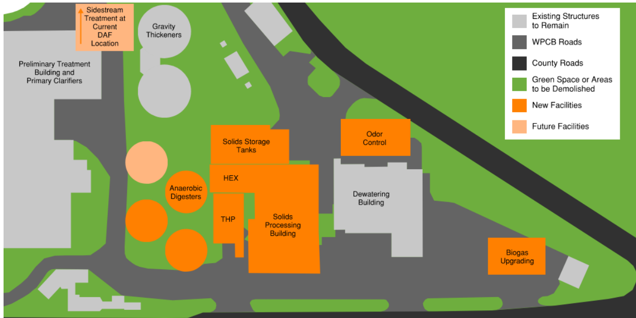
Figure 17-3. Option 2: Decommission Existing Dewatering Building—Alternative Concept 2
