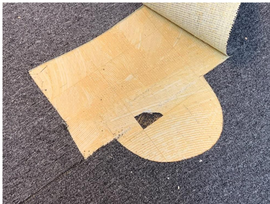
Homogeneous Material No. 18 – ACM 9" by 9" White Vinyl Floor Tile with Black Mastic located in the Building Mezzanine Floor, Office Space of the Subject Property
