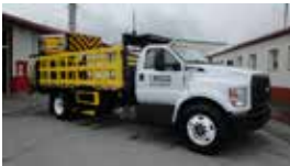
Truck w/Arrow Board & Attenuator
