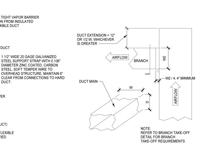
**DUCT EXTENSION = 12"** OR 1/2 W, WHICHEVER IS GREATER -**DUCT MAIN -**REFER TO BRANCH TAKE-OFF DETAIL FOR BRANCH TAKE-OFF REQUIREMENTS **REFER TO BRANCH TAKE-OFF** DETAIL FOR BRANCH **DESIGNER NOTES:** TAKE-OFF REQUIREMENTS **DESIGNER NOTES:** USE WHERE "W" EXCEEDS 24" OR WHEN USE WHERE "W" IS LESS THAN 24", WHEN YOU AIR FLOW IS IN EXCESS OF 1500 CFM. HAVE ROUND DUCT BRANCHES TO DIFFUSERS.
