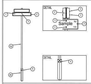
Install Street Name Signs on Corners Of Intersection so that they will be on the Far Right Side on the Intersection for Traffic on the Major Street in accordance with MUTCD Section 2D.38
