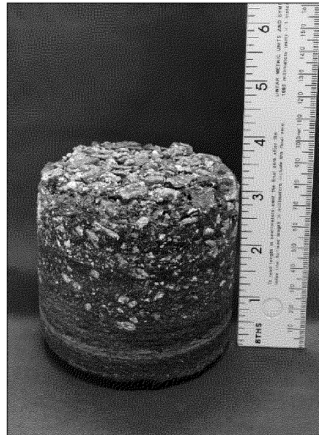
Boring P-13 Located at (30.924973°, -86.539868°) total thickness of 3 3/8 inches.
