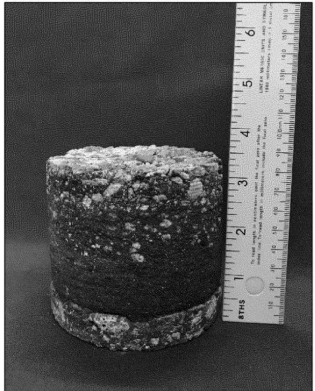
Boring P-10 Located at (30. 925209°, -86. 564592°), total thickness of 3 3/8 inches.
