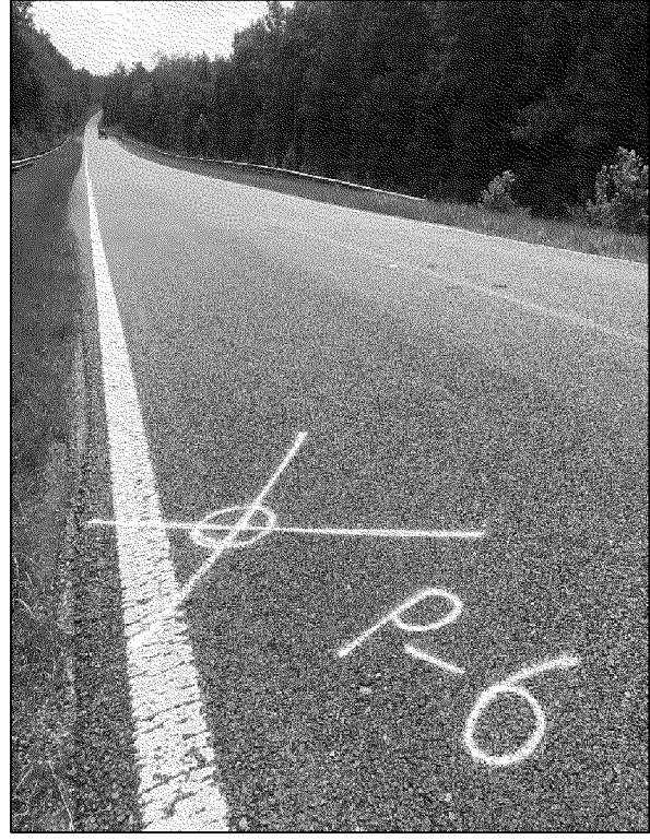
Boring P-6 Located at (30. 922711°, -86. 594893°), total thickness of 4 inches.
