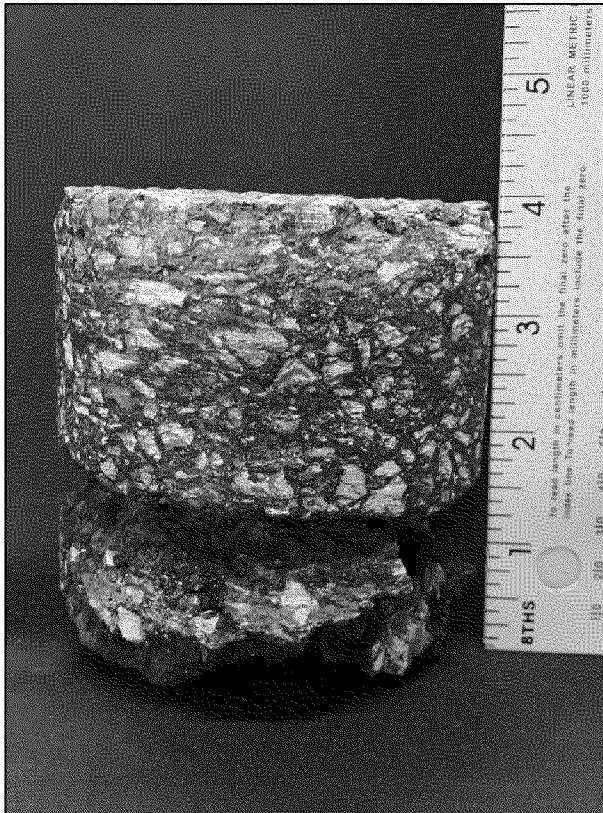
Boring P-6 Located at (30. 922711°, -86. 594893°), total thickness of 4 inches.
