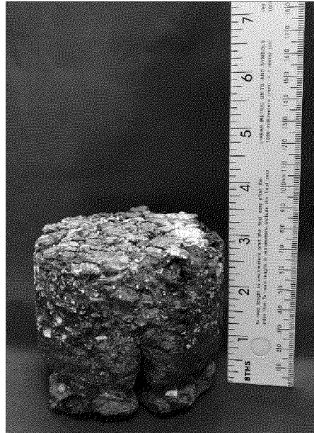
Boring P-17 Located at (30. 924581°, -86. 507425°), total thickness of 4 3/8 inches.
