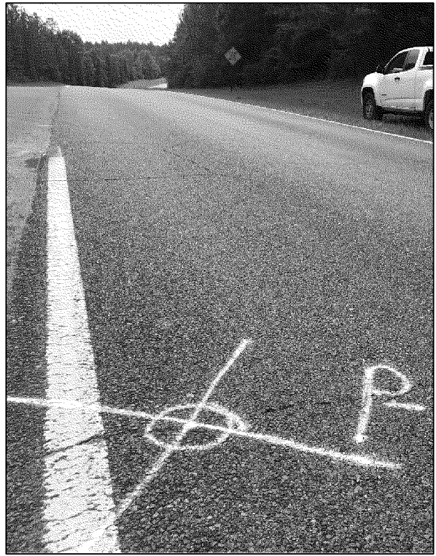
Boring P-5 Located at (30. 918035°, -86. 601606°), total thickness of 3 3/4 inches.
