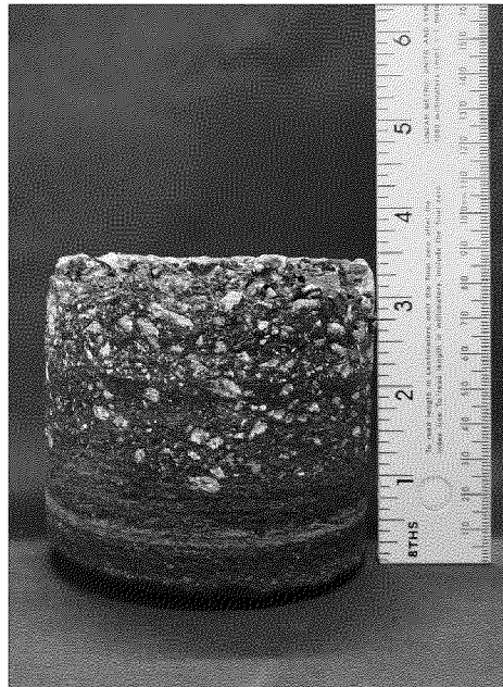
Boring P-13 Located at (30.924973°, -86.539868°) total thickness of 3 3/8 inches.
