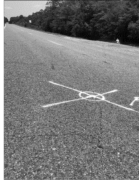
Boring P-11 Located at (30. 925176°, -86. 555313°), total thickness of 2 ½ inches.
