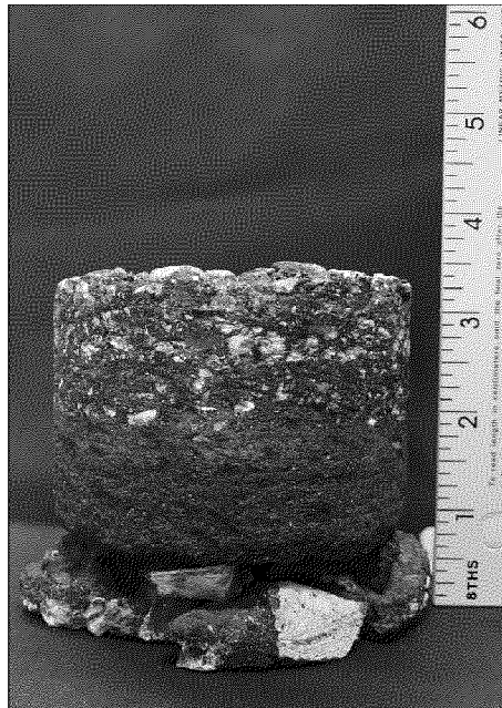
Boring P-4 Located at (30. 917737°, -86.609594°), total thickness of 3 7/8 inches.
