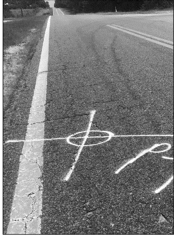
Boring P-15 Located at (30. 924761°, -86. 523579°), total thickness of 2 3/4 inches.
