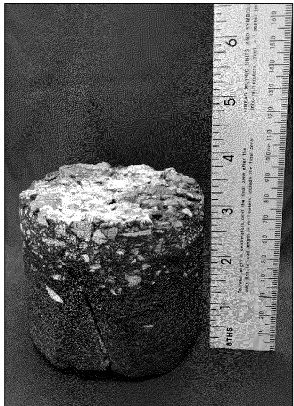
Boring P-19 Located at (30. 924418°, -86. 490987°), total thickness of 3 1/8 inches.
