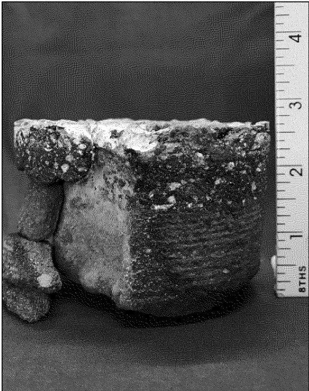
Boring P-15 Located at (30. 924761°, -86. 523579°), total thickness of 2 3/4 inches.
