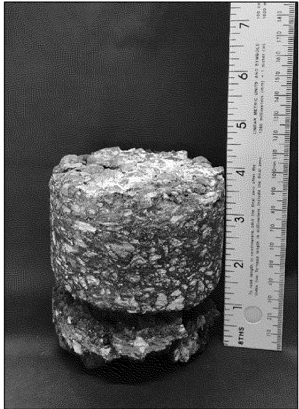
Boring P-6 Located at (30. 922711°, -86. 594893°), total thickness of 4 inches.
