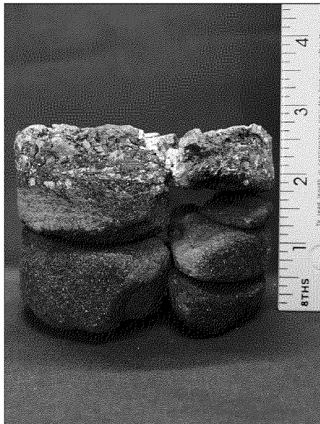
Boring P-1 Located at (30.924767°, -86.632324°), total thickness of 2 3/4 inches.
