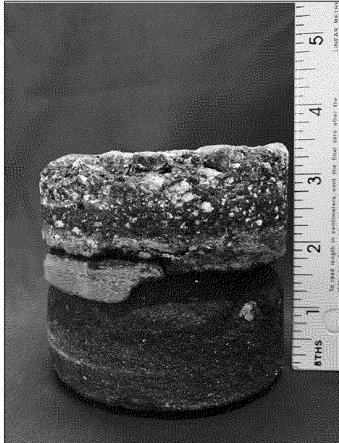
Boring P-18 Located at (30. 924498°, -86. 499137°), total thickness of 3 3/8 inches.
