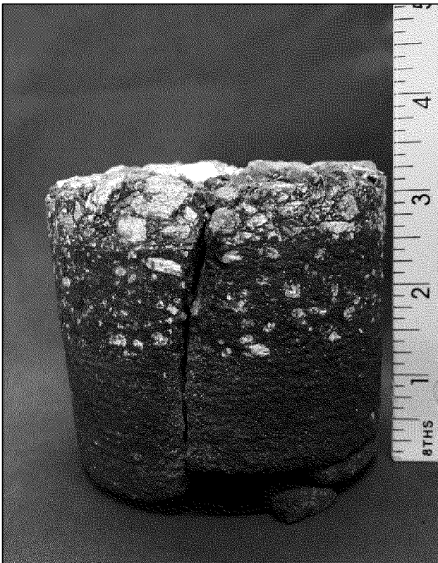
Boring P-20 Located at (30. 924296°, -86. 483084°), total thickness of 3 ¼ inches.
