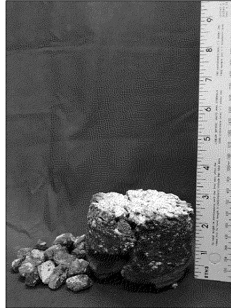
Boring P-11 Located at (30. 925176°, -86. 555313°), total thickness of 2 ½ inches.
