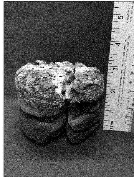
Boring P-1 Located at (30.924767°, -86.632324°), total thickness of 2 3/4 inches.
