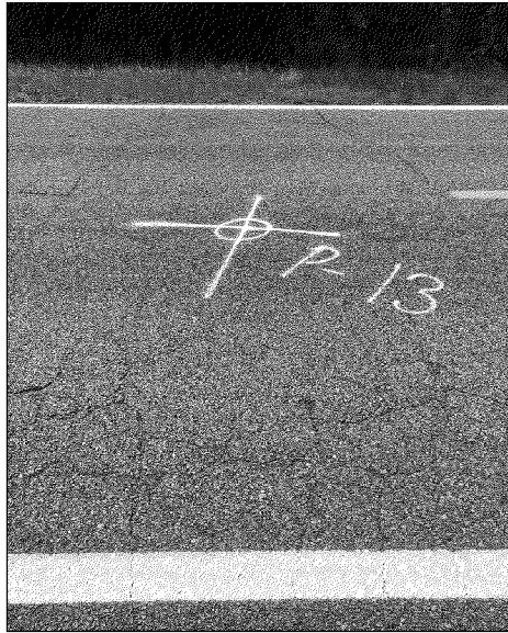
Boring P-13 Located at (30. 924973°, -86. 539868°) total thickness of 3 3/8 inches.
