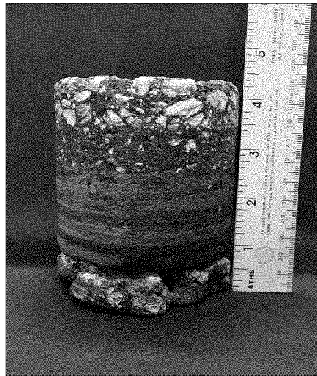
Boring P-14 Located at (30. 924897°, -86. 531723°), total thickness of 4 3/8 inches.
