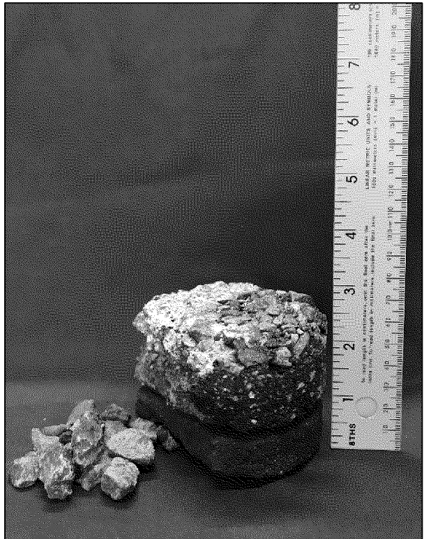
Boring P-12 Located at (30. 925120°, -86. 548012°), total thickness of 5 7/8 inches.
