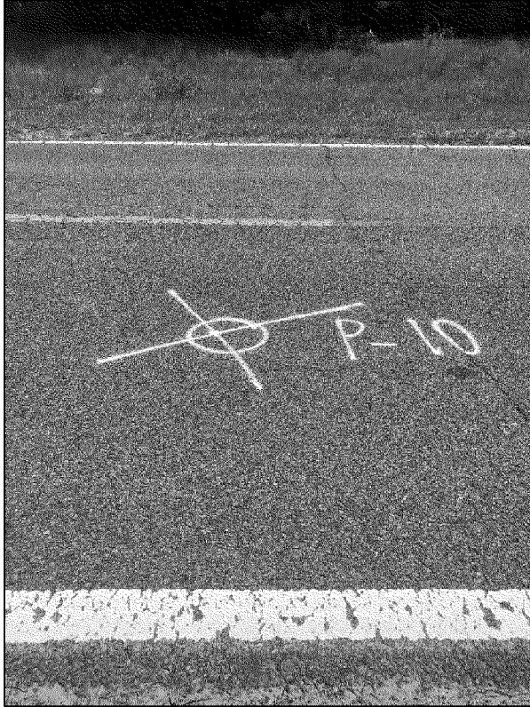
Boring P-10 Located at (30. 925209°, -86. 564592°), total thickness of 3 3/8 inches.
