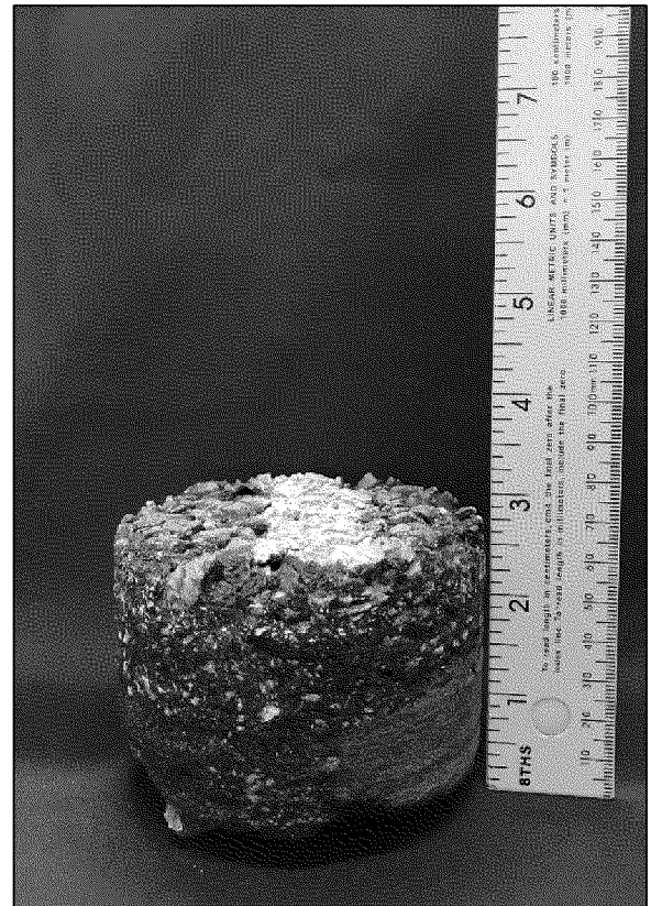
Boring P-16 Located at (30. 924669°, -86. 515431°), total thickness of 2 ¾ inches.
