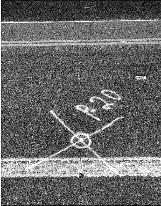
Boring P-20 Located at (30. 924296°, -86. 483084°), total thickness of 3 ¼ inches.
