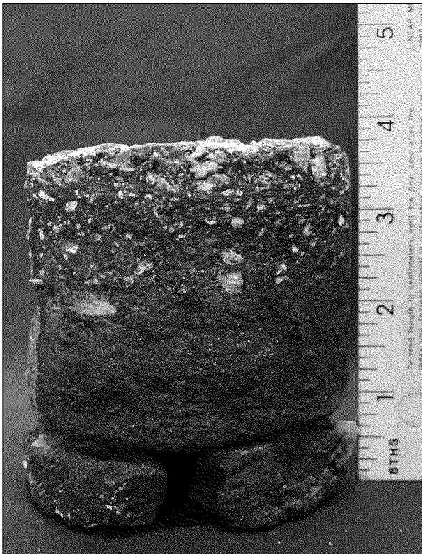
Boring P-5 Located at (30. 918035°, -86. 601606°), total thickness of 3 3/4 inches.
