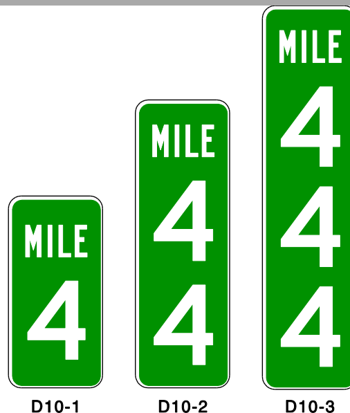
Figure 2H-2. Reference Location Signs*
