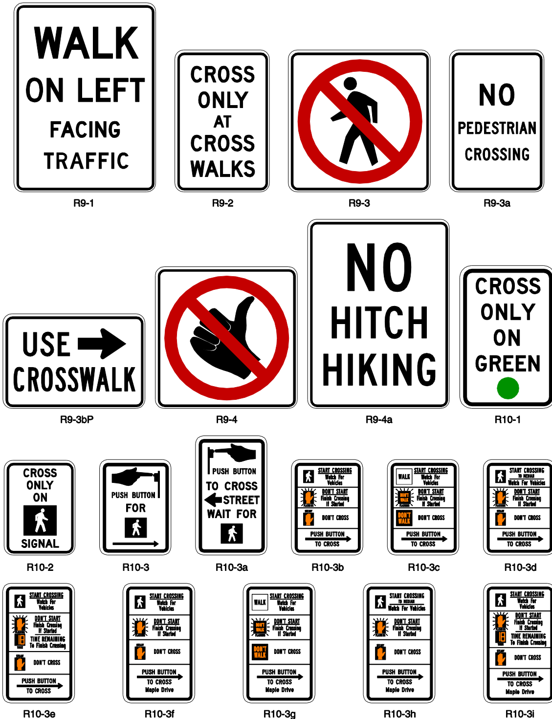
Figure 2B-26. Pedestrian Signs and Plaques (Sheet 1 of 2)
