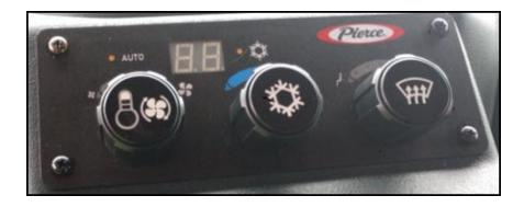
The system will control the temperature of the cab and crew cab automatically by pushing the center of the fan speed control knob. Rotate the center temperature control knob to set the cab and crew cab temperature.
