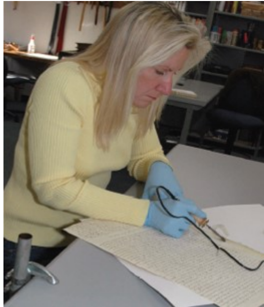
Kofile carefully coaxes adhesives and tape with mechanical application of heat and pressure.
